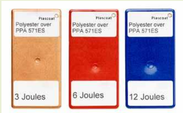
▲ A 1mm plate coated in Plascoat® PPA 571 and polyester after an impact of up to 12 Joules.
